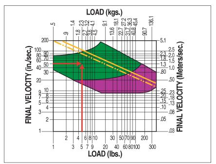
In the following example, the cylinder is carrying a 10 lb load and traveling at a final velocity of 80 inches per second when coming in contact with the shock absorber located at the ends of the cylinder stroke. The load must be stopped within the shock absorber stroke of 0.50 inches. The Mz and equivalent force applied to the cylinder's load carrying device need to be within the limits of the cylinder's rating capacities.
