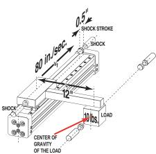
$a \times P = 6400 \text{ in/sec}^2 \times 10 \text{ lbs} = 165.6 \text{ lbs}$ g 386.4 in/sec<sup>2</sup>
