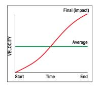
Velocity calculations for all rodless cylinders need to differentiate between average velocity and impact velocity.
