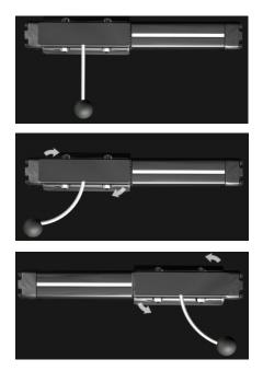
In the first illustration, the ball represents an overhung side load exerting a Mx moment on the cylinder's carrier.
